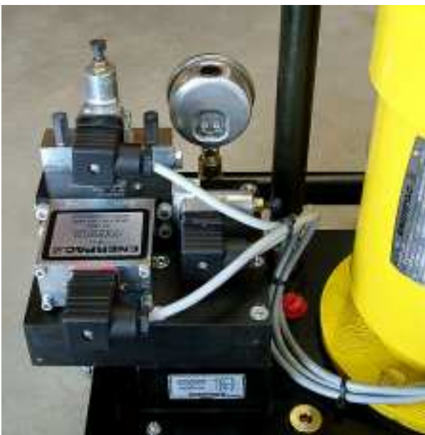
photo 3: electrical connectors for isolating valve pump's pressure switch 100 - 350 bar,
